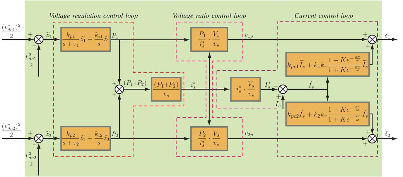
Fig. 10. Block diagram of the system controller.
