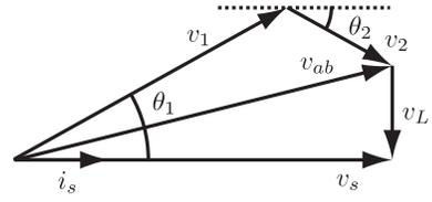
Fig. 3. 2C-CHB phasorial diagram of voltages and current.
