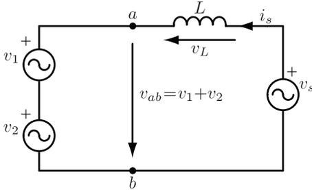
Fig. 2. 2C-CHB equivalent circuit.
