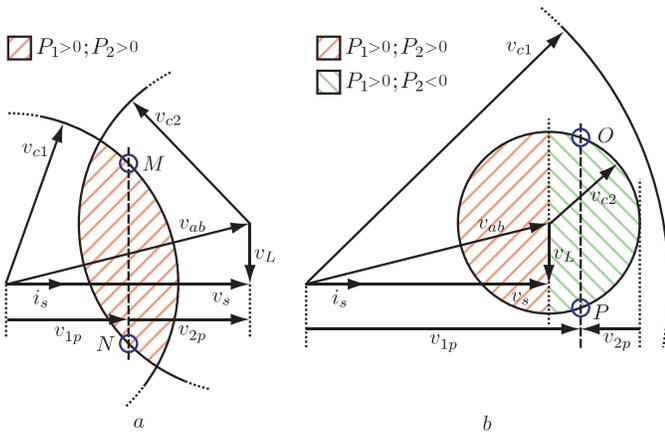
Fig. 11. Set of possible solutions for a particular active power distribution. From left to right: a)  $v_{c1} \leq v_{ab}$  and  $v_{c2} \leq v_{ab}$ . b)  $v_{c1} > v_{ab}$  and  $v_{c2} \leq v_{ab}$ .
