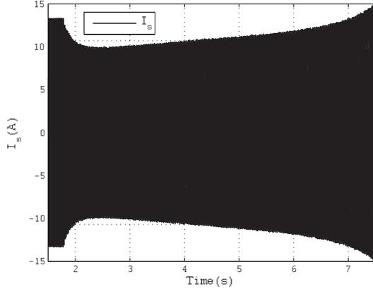
Fig. 16. Evolution in time of grid current.
