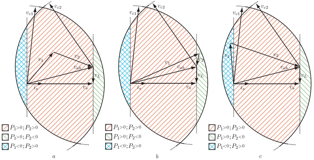
Fig. 8. Stable control area when  $v_{c1} > v_{ab}$  and  $v_{c2} > v_{ab}$ . From left to right: Possible solution with: a)  $P_1 > 0$  and  $P_2 > 0$ . b)  $P_1 > 0$  and  $P_2 < 0$ . c)  $P_1 < 0$  and  $P_2 > 0$ .
