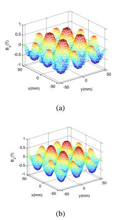
Fig.8. Air-gap flux density distribution. (a) Analytical result. (b) FE result.
