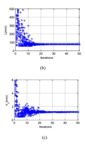
Fig.15. The positions of the particles. (a) Pole pitch. (b) Length of the windings. (c) Thickness of the windings.
