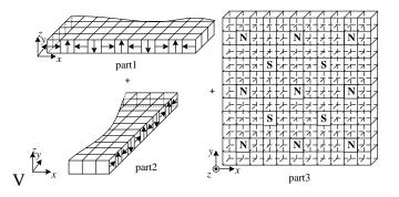
Fig.4. Decomposition of the PM array.
