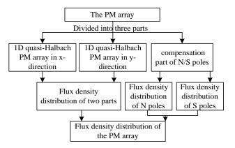
Fig.5. Overall diagram of the analytical model.
