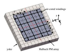
Fig.1. Topology of the planar motor.
