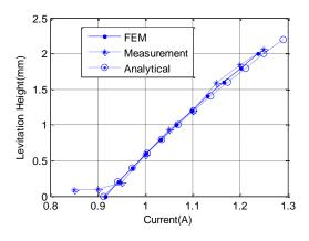
Fig.18. Relationship between levitation height and current.
