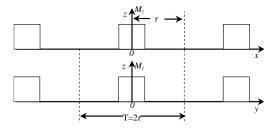
Fig.7. Magnetization distribution of N poles.
