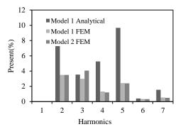
Fig.10. Comparison of the harmonics in  $B_{zav}$ (airgap=2mm).
