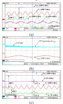
Fig. 9. Experimental results (inversion mode): (a) Voltages  $V_{DC}$  and  $V_{-}$ , grid voltage  $v_g$  and current  $i_g$ ; (b) CM voltage  $v_{D_NN}$  and its spectra; (c) Voltages  $V_{DC}$  and  $V_{-}$ , DC-bus current I and capacitor current  $i_{C-}$  after applying a 6 kHz low-pass filter to remove the switching ripples.
