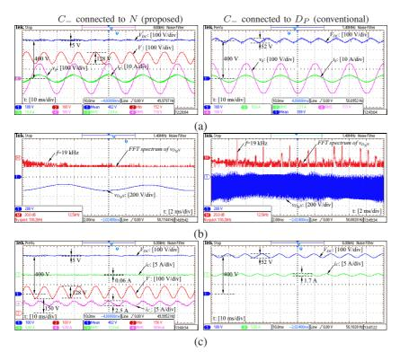
Fig. 6. Experimental results at the steady state (rectification mode): (a) Voltages  $V_{DC}$  and  $V_{-}$ , grid voltage  $v_g$  and current  $i_g$ ; (b) CM voltage  $v_{D_NN}$  and its spectra; (c) DC voltages  $V_{DC}$  and  $V_{-}$ , capacitor currents  $i_C$  and  $i_{C-}$  after applying a 6 kHz low-pass filter.
