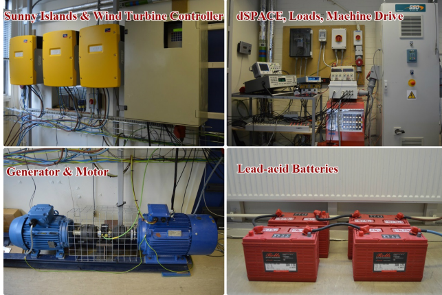
Fig. 9. Hybrid system lab setup equipment
