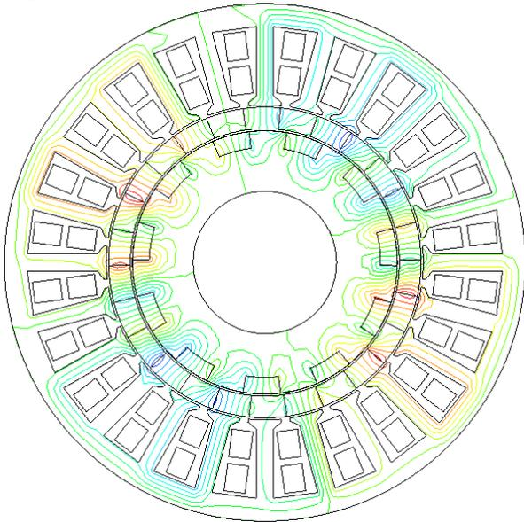
Fig. 9. The no-load flux-line distribution of the optimal DF-BFM.
