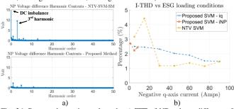
Fig. 26. Processed experimental results a) FFT of NP voltage difference for both methods b) AC-side current THD for NTV-SVM and proposed SVM  $\,$
