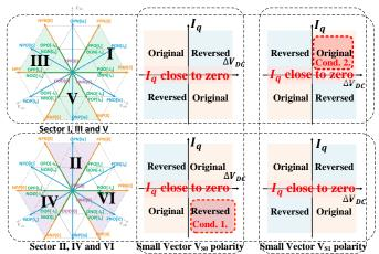
Fig. 13. Small vector polarity selection - Iq method
