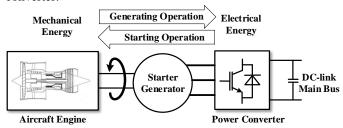
Fig. 1. Diagram of the target starter generator system
