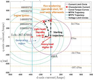
Fig. 4. Operating trajectory of the target system
