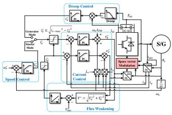
Fig. 3. Control structure for the target ESG system [28]
