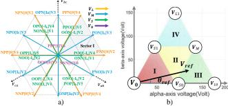
Fig. 5. Conventional SVM strategy a) space vector diagram for NPC converter b) space vector diagram in sector I
