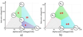
Fig. 16. Number of commutations per switching period for a) NTVV-SVM method b) the proposed method in medium to high modulation region
