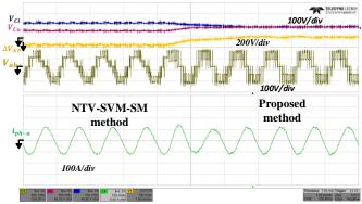
Fig. 25. Transition from NTV-SVM-SM to proposed SVM at light load (iq = -15A, Averaged MI = 0.912, Averaged PF = 0.137)
