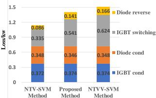
Fig. 21. Converter loss comparison when ESG is on standby mode at 20krpm
