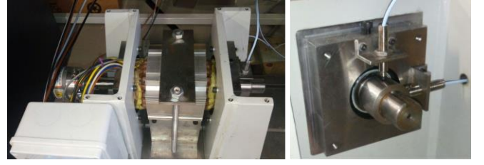
Fig. 5 – Prototype of bearingless multi-sector permanent magnet machine (left) and x-y displacement sensors (right).
