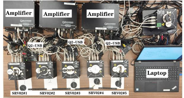
Fig. 8. The experimental system with five heterogeneous SRV02.
