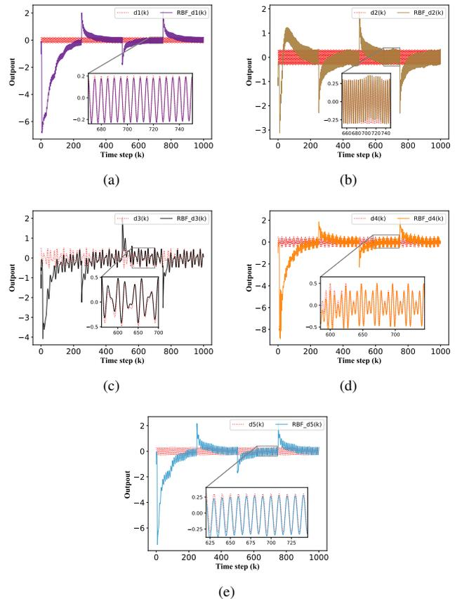
Fig. 5. Performances of the designed online learning RBFNN disturbance observers in Example 2: (a), (b), (c), (d), and (e) are disturbances estimation of five agents, respectively.
