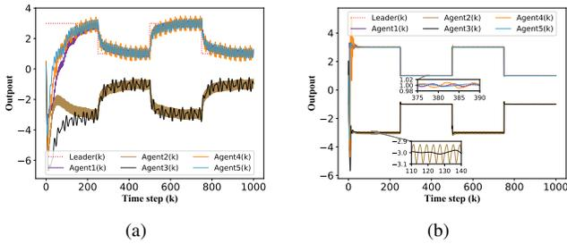
Fig. 6. Bipartite consensus control performances of the MASs with unknown disturbances in Example 3: (a) Without the RBFNN disturbance observer; (b) With the RBFNN disturbance observer.
