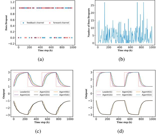
Fig. 4. Bipartite consensus control for the MASs without disturbance in Example 1: (a) Random data loss; (b) The numbers of consecutive data losses; (c) Without input compensation; (d) With input compensation.
