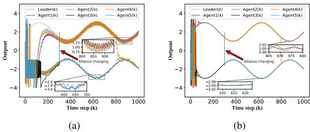
Fig. 7. Bipartite consensus performances of the MASs with time-varying trajectory and switching topologies in Example 4: (a) The existing method [34]; (b) The designed LRBC method.
