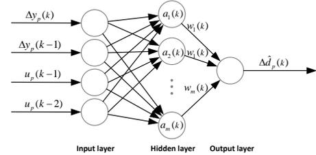
Fig. 2. The diagram of the designed RBFNN disturbance observer.
