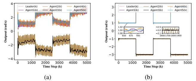
Fig. 9. Performances of bipartite consensus with five SRV02 in Example 5: (a) The designed LRBC method without the RBFNN disturbance observer; (b) The designed LRBC method with the RBFNN disturbance observer.
