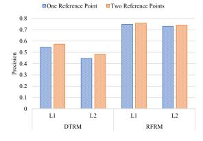
Fig. 9. System precision with one and two reference points calibration
