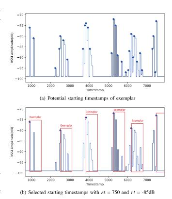
Fig. 3. Exemplar timestamp is detected in RSSI sequence collected from one reference point. The sensitivity is set to -99dB since RSSI lower than this threshold occurs from a remote beacon.
