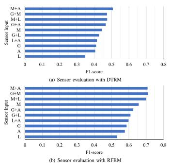
Fig. 10. Performance results in descending order for different sensors: Gyroscope (G), Magnetic Field Sensor (M), Linear Acceleration Sensor (L), Accelerometer (A)
