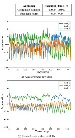
Fig. 5. Turning event is more evident after filtering movement noises
