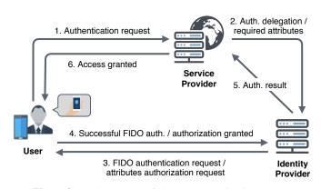
Figure 3: FIDO-enhanced federated authentication process.
