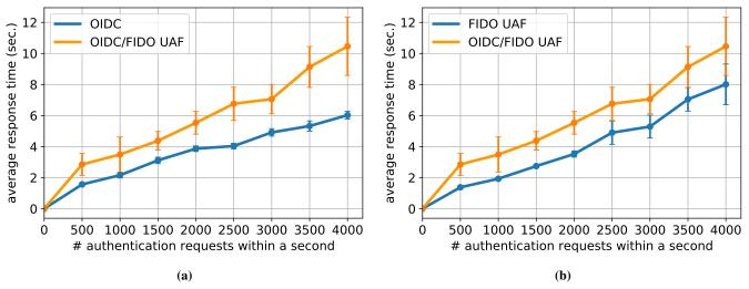
Figure 5: Average response time of an OIDC/FIDO UAF authentication request compared with vanilla: (a) OIDC authentication request; and (b) FIDO UAF authentication request.
