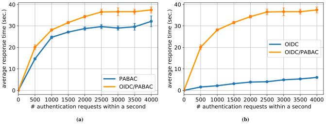
Figure 6: Average response time of an OIDC/PABAC authentication request compared with vanilla: (a) Idemix authentication request; and (b) OIDC authentication request.
