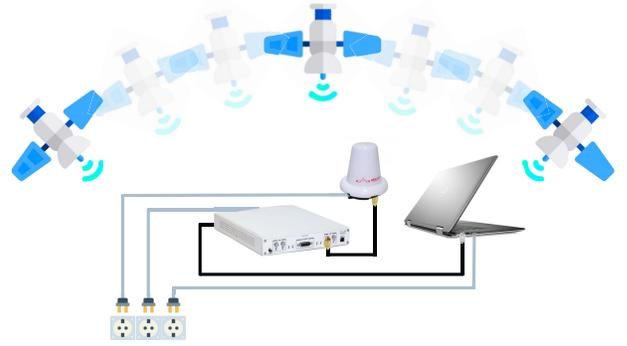
Fig. 3. Measurement Setup: we adopted an active (pre-amplified) Iridium antenna (Beam RST740) connected to a USRP X310 Software Defined Radio.
