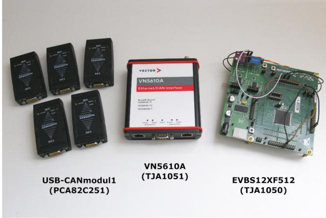
Figure 10: CAN bus prototype.
