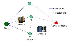
Fig. 1. An industrial WSN consisting of a sink and N sensors in the presence of an eavesdropper (e).
