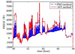
Fig. 8. Power output of HESS with PSO and with AIT
