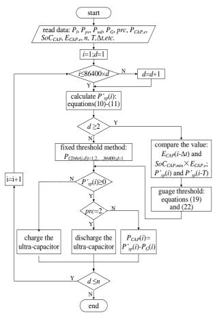
Fig. 2. Algorithm for ultra-capacitor Management System
