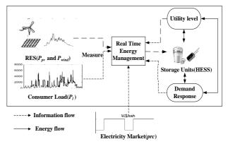
Fig. 1. Structure of Energy Management System
