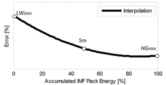
Fig. 3. Example of a resulting error threshold curve in regard with the accumulated energy,  $R_e$ , of the IMF package. The curve is described by the interpolation of a second order function within the three points defined,  $LW_{MAX}$ ,  $S_m$  and  $HG_{MAX}$ .
