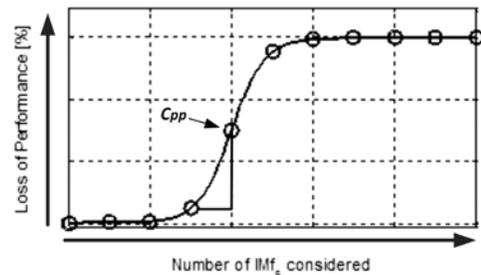
Fig. 2. Representation of the effect over the resulting accumulated error of the number of IMF considered for a single model. The critical performance point,  $C_{pp}$ , represents an allowable down limit in regard with the modelling performance. This curve is obtained by the successive evaluating of the IMFs extracted from multi-sinus signal of 11 frequencies in a classic 1-input 1-output ANFIS structure at a forecasting horizon of 10 samples.
