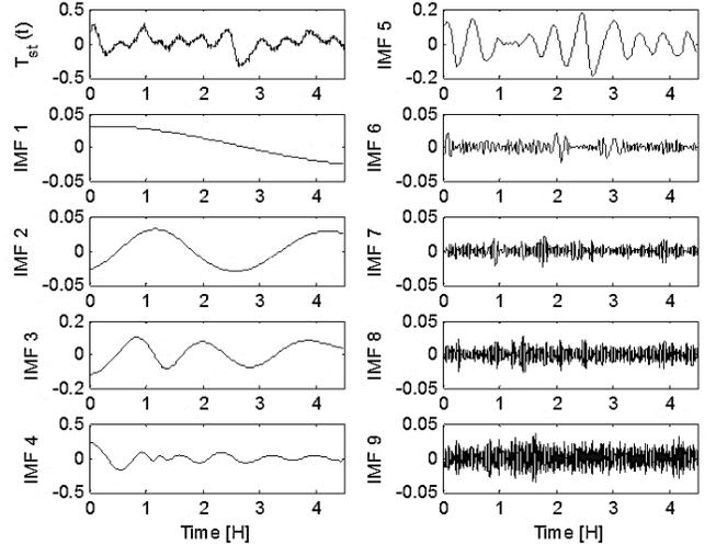
Fig. 7. Intrinsic mode functions extracted from the tundish's temperature of the training set during a time window processing.
