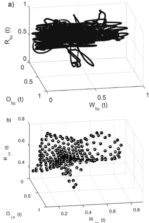
Fig. 10. a) SOM input data space of training set: x) Tundish's Oxygen value in ppm, y) Tundish burner's ratio in % and z) Copper weight in the tundish in Kg. b) Neurons of the SOM grid after the training procedure.
