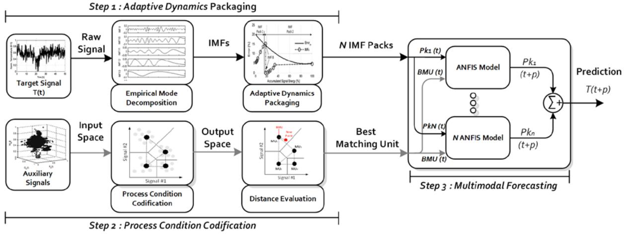
Fig. 1. Block diagram of the design procedure of the proposed multimodal modelling method. The procedure is divided in three steps: (i) Adaptive dynamics packaging, (ii) Process condition codification, and (iii) Multimodal forecasting.
