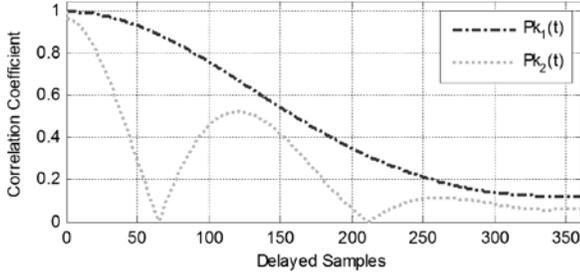
Fig. 12. Autocorrelation analysis between the IMF packages ( $Pk_1$  and  $Pk_2$ ), and their successive delayed signals.
