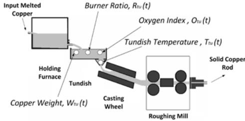
Fig. 5. Diagram of the copper rod manufacturing process [22].
