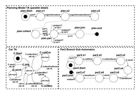
Fig. 5. Generated TA structure
