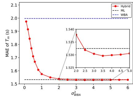
Fig. 10. Effect of  $\sigma_{WBA}^2$  on the estimation error of the mean wave period.
