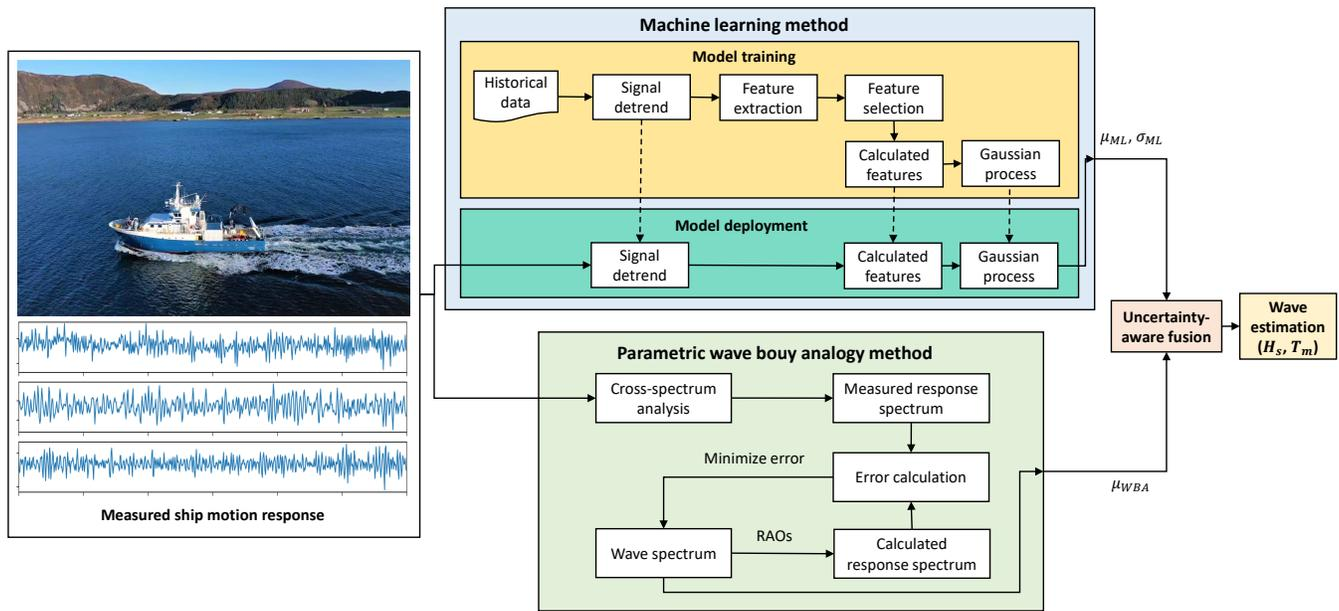
Fig. 1. Schematic illustration of the proposed hybrid approach. The upper rectangle is the ML model and the lower rectangle is the model-based method.
