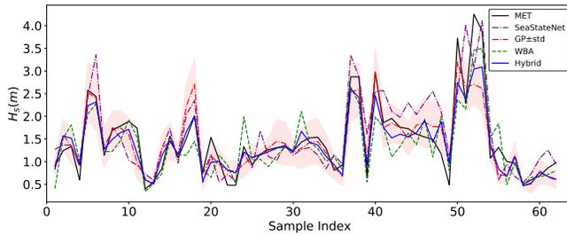
Fig. 11. Estimation of significant wave height by different approaches.
