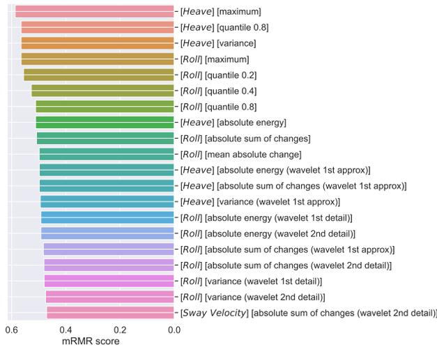
Fig. 7. Features ranked by mRMR criterion for significant wave height.
