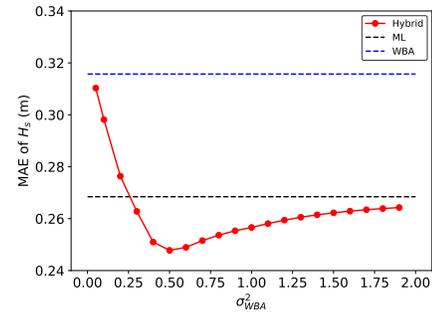
Fig. 9. Effect of  $\sigma_{WBA}^2$  on the estimation error of the significant wave height.
