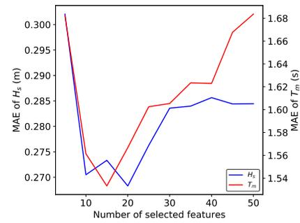
Fig. 6. Number of selected features VS. MAE of significant wave height and mean wave period.
