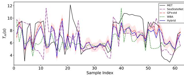
Fig. 12. Estimation of mean wave period by different approaches.
