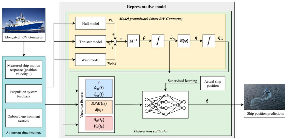
Fig. 1: A complete flowchart showing the incorporating of approximate dynamics into the data-driven calibrator.
