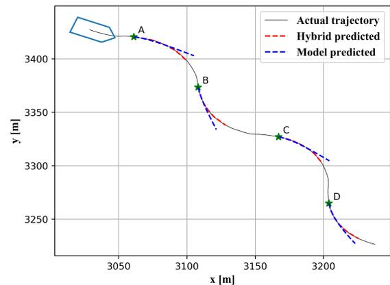
Fig. 10: Hybrid predictions in comparison with model predictions in real life.
