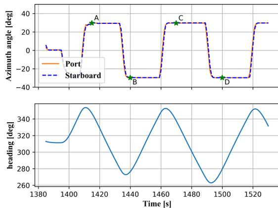
Fig. 9: Azimuth turning angle and ship heading during maneuvering.
