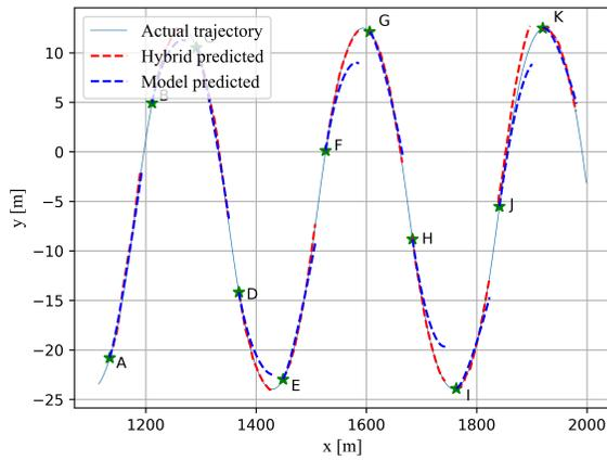
(a) Predicted ship positions of model-based and hybrid approach
