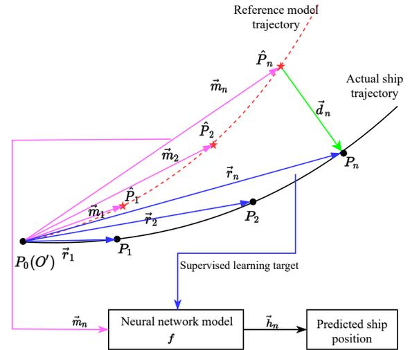
Fig. 2: Illustration of the data-driven calibration concept.
