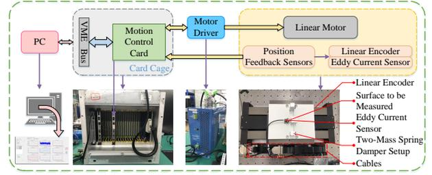
Fig. 6: Block diagram of the experimental setup.
