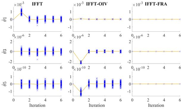
Fig. 4: Parameter  $[\hat{\theta}_1, \hat{\theta}_3, \hat{\theta}_5]$  as a function of iteration for  $M = 100$  realizations for IFFT (left), IFFT-OIV (middle) and IFFT-FRA (right). Their ideal results are thought to infinitely approximate to  $\mathbf{0}$ .
