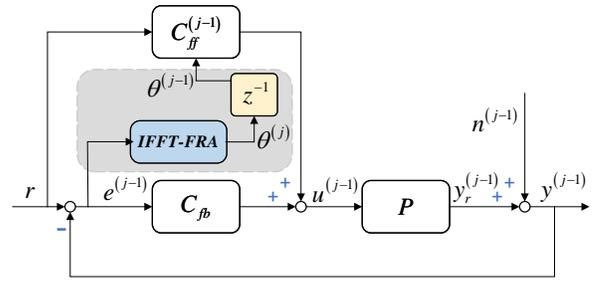
Fig. 1: Two-degrees-of-freedom control configuration with IFFT-FRA tuning algorithm. The symbol  $z$  denotes the forward shift operator with respect to iteration and the superscript  $j$  denotes the iteration index.
