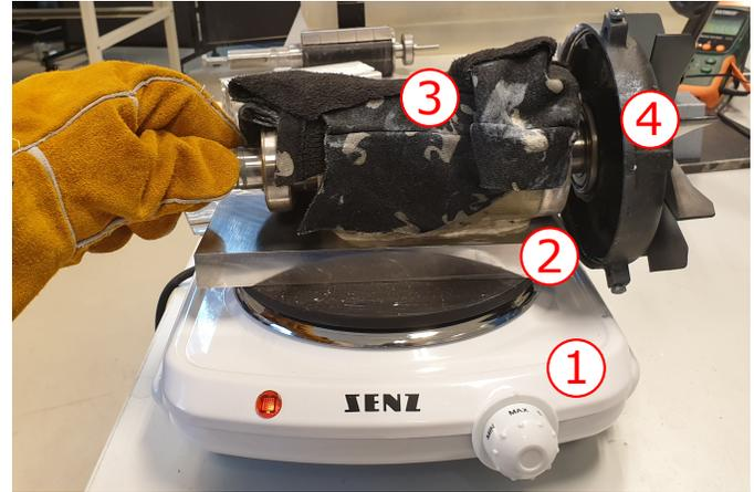
Fig. 6. Thermal treatment setup consisting of (1) cooking plate, (2) solid aluminium block, (3) wet towel and (4) the motor end shield
