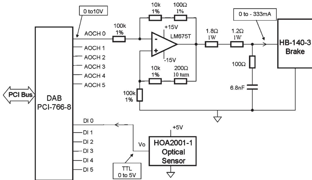
Fig. 6. Interface electronics between the DAB and one of the exercise stations.
