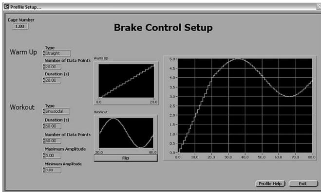
Fig. 8. GUI used to setup load torque profiles.
