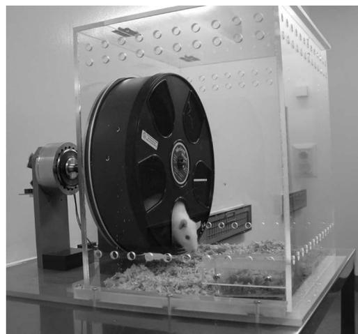
Fig. 4. Front view of a rat exercise station showing a rat using the wheel.
