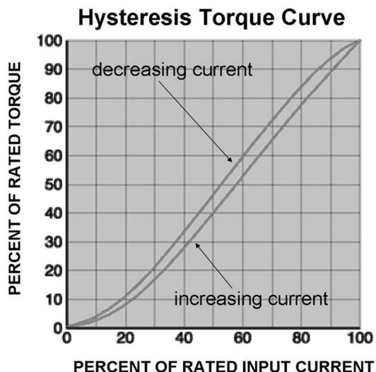
Fig. 2. Typical hysteresis characteristic (reproduced from Placid Industries, Inc. [6]).
