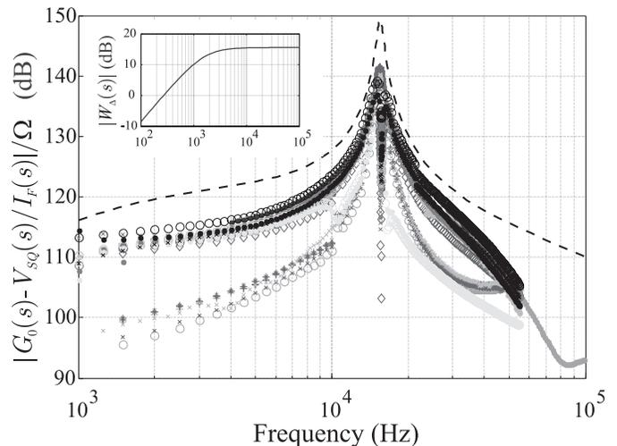
Fig. 6. Absolute value of the differences between the nominal model and the experimental data. The results are covered by the proposed dynamic uncertainty weight multiplied by the nominal model,  $G_0(s) \cdot W_\Delta(s)$  (black dashed line). Inset:  $W_\Delta(s)$ .
