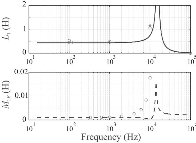
Fig. 3. Measurement results of  $L_1$  and  $M_{1F}$ , in the top and bottom figures, respectively. The values at cryogenic (red star) and ambient (red circle) temperatures are shown. The simulations for the self-inductance at 4.2 K (blue solid line) and the mutual inductance at 300 K (blue dashed line) are also presented.
