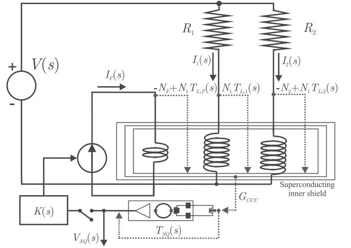
Fig. 2. Schematic of the two-terminal CCC. The notation for the transfer functions from the origin to the end of the blue-dotted arrows is indicated. In the feedback loop, a switch is included to indicate where the loop is opened.
