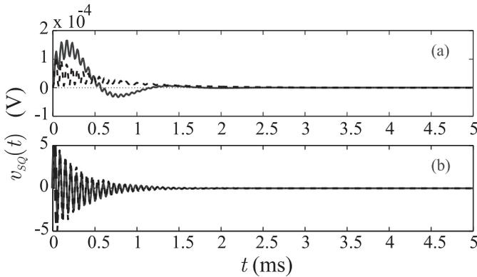
Fig. 9. (a) Step and (b) impulse simulated responses of the closed-loop system for the identified model (black dashed line) and the worst case model (blue solid line). The excitation amplitudes were 0.1 pA in the primary winding in both cases.
