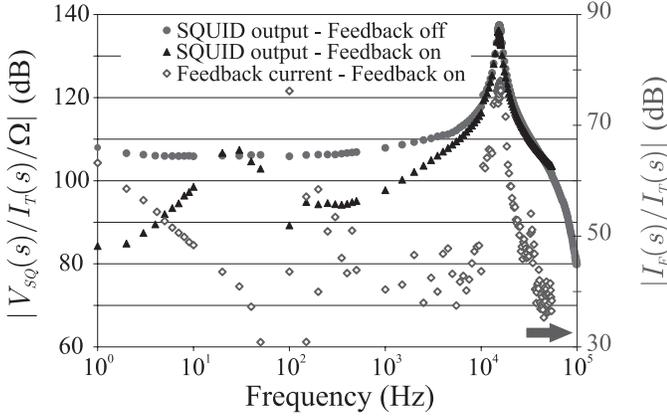
Fig. 1. Absolute value of the frequency response measurements of the SQUID voltage from a test current  $I_T(s)$  in a single-turn winding, with integral feedback OFF (red circle) and ON (black triangle). The response of the feedback current from the same input in closed loop is shown in the secondary axis (blue diamond).
