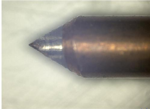
Figure 2.15 Sharpened micro-coaxial tip.
