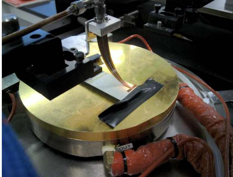
Figure 3.10 Printed loop probe with integrated balun scanning the sample.
