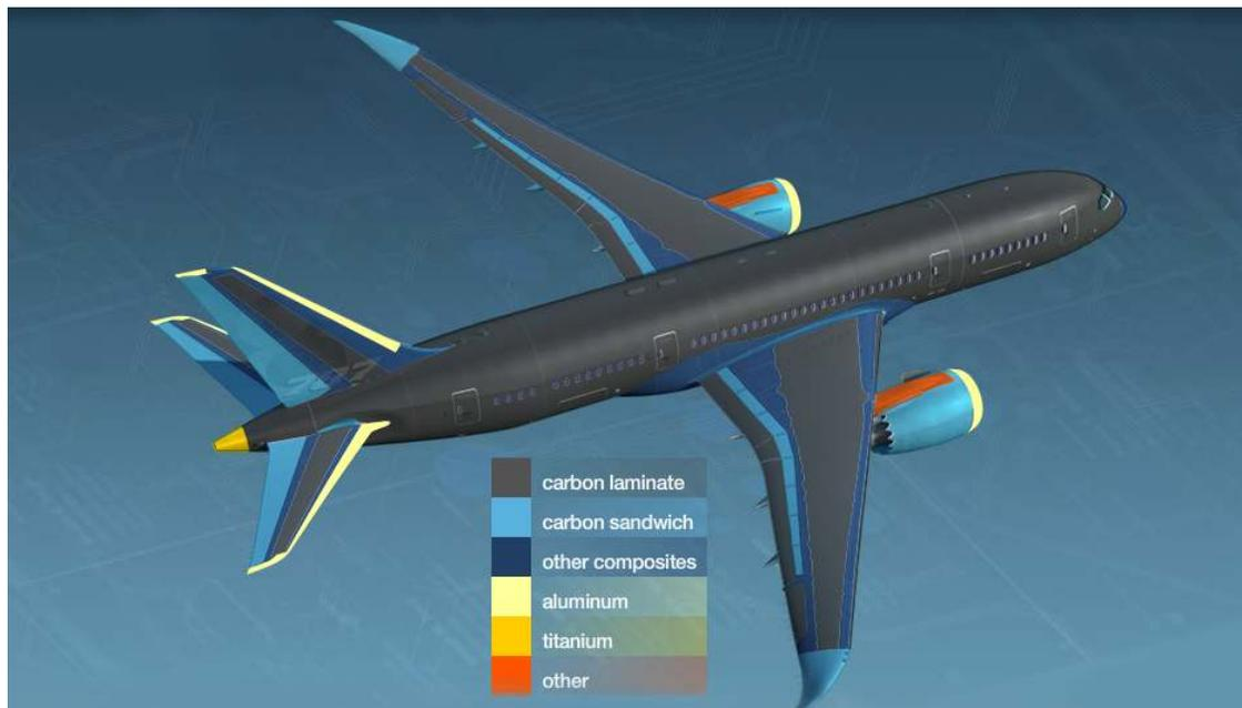
Figure 1.1 Composites are used in more than 50% of the *Boeing 787* aircraft fuselage [1].
