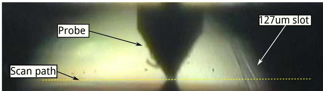
Figure 2.16 Sharpened micro-coaxial tip scanning 127  $\mu\text{m}$  width slot
