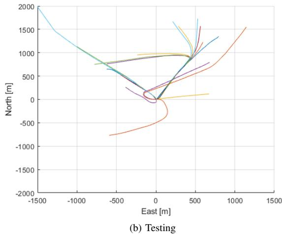
Fig. 4. The North-East path taken by the RV Gunnerus for all docking operations used in this study.
