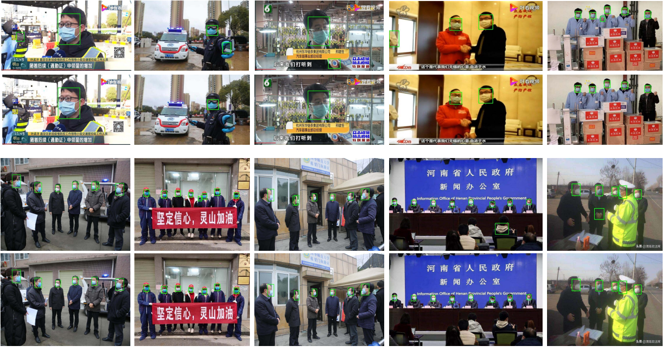
Fig. 7. Visual comparison between Faster_RCNN-InceptionV2 and ours. The first and third rows are generated by Faster_RCNN-InceptionV2, and the second and the fourth rows are generated by our approach.
