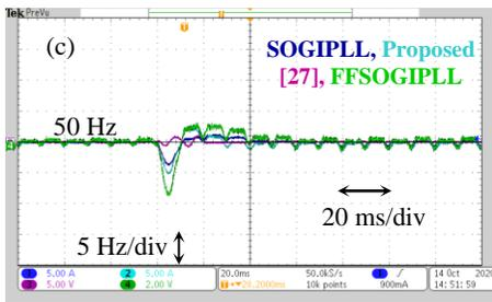
Fig. 13. Frequency dynamics with 2% 3<sup>rd</sup> and 5<sup>th</sup> harmonics during (a) +1 Hz Frequency variations (b) -45° PAJ and (c) 50% sag. (PLL settling time = 120 ms and  $k_{SOGI} = 1.414$ ): Ch-1: SOGIPLL, Ch-2: Proposed, Ch-3: ref [27], Ch-4: FFSOGIPLL.
