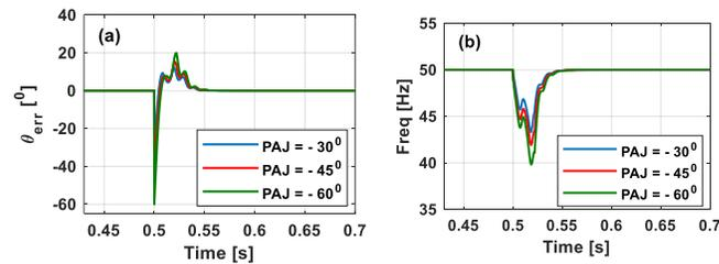
Fig. 7. (a) Phase-angle error and (b) Frequency dynamics with [27] during the combination of 50% voltage sag and various PAJs.
