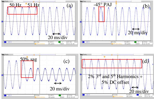
Fig. 10. Grid voltage disturbances: (a) +1 Hz Frequency variations, (b)  $-45^\circ$  PAJ and (c) 50% sag, and (d) Harmonics (2% 3<sup>rd</sup> and 5<sup>th</sup>) + 5% DC offset.
