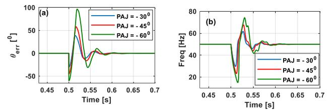
Fig. 5. (a) Phase-angle error and (b) Frequency dynamics with fast SOGIPLL ( $t_s = 60$  ms) during the combination of 50% voltage sag and various PAJs.
