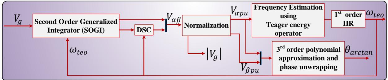
Fig. 2. Proposed frequency-adaptive SOGI based grid synchronization technique.
