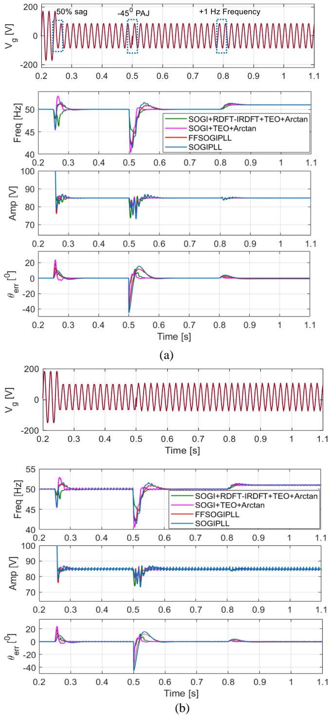
Fig. 4. Grid synchronization dynamics comparison during 50% sag at  $t = 0.25$  s,  $-45^\circ$  PAJ at  $t = 0.5$  s and +1 Hz frequency variations at  $t = 0.8$  s: (a) with undistorted grid voltage, (b) with grid voltage distortion having 5% DC offset and harmonics (5% THD).
