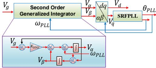
Fig. 1. Grid synchronization using SOGIPLL technique.
