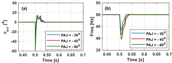
Fig. 8. (a) Phase-angle error and (b) Frequency dynamics with the proposed technique during the combination of 50% voltage sag and various PAJs.
