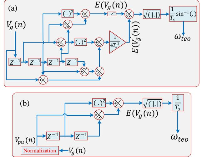
Fig. 3. Frequency estimation of grid voltage ( $V_g$ ) using teager energy operator in discrete domain: (a) actual model and (b) simplified model.
