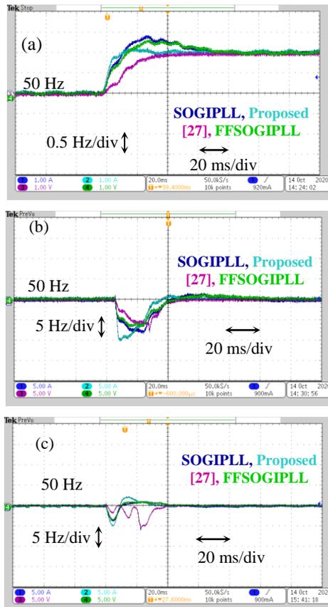
Fig. 11. Frequency dynamics during (a) +1 Hz Frequency variations (b)  $-45^\circ$  PAJ and (c) 50% sag. (PLL settling time = 120 ms): Ch-1: SOGIPLL, Ch-2: Proposed, Ch-3: ref [27], Ch-4: FFSOGIPLL.
