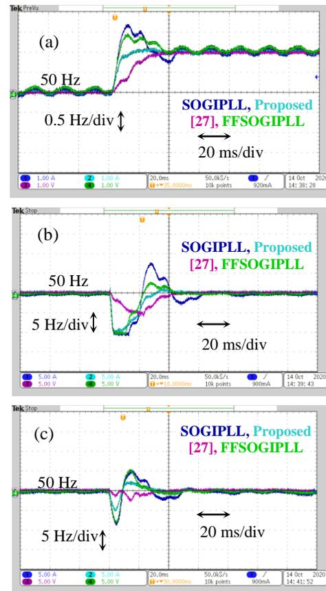
Fig. 12. Frequency dynamics during (a) +1 Hz Frequency variations (b)  $-45^\circ$  PAJ and (c) 50% sag. (PLL settling time = 60 ms): Ch-1: SOGIPLL, Ch-2: Proposed, Ch-3: ref [27], Ch-4: FFSOGIPLL.
