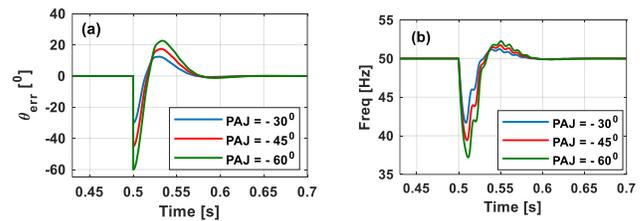
Fig. 6. (a) Phase-angle error and (b) Frequency dynamics with slow SOGIPLL ( $t_s = 120$  ms) during the combination of 50% voltage sag and various PAJs.
