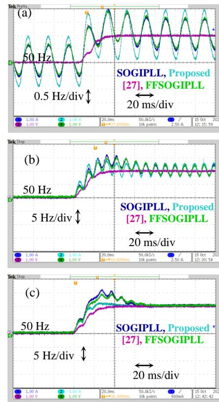
Fig. 15. Impact of addition of 5% DC offset in the grid voltage on frequency estimation: (a) no use of DSC, (b) use of fixed frequency DSC, and (c) use of frequency-adaptive DSC: Ch-1: SOGIPLL, Ch-2: Proposed, Ch-3: ref [27], Ch-4: FFSOGIPLL.
