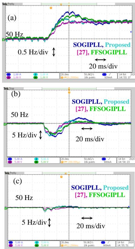
Fig. 14. Frequency dynamics with 2% 3<sup>rd</sup> and 5<sup>th</sup> harmonics during (a) +1 Hz Frequency variations (b) -45° PAJ and (c) 50% sag. (PLL settling time = 120 ms and  $k_{SOGI} = 0.707$ ): Ch-1: SOGIPLL, Ch-2: Proposed, Ch-3: ref [27], Ch-4: FFSOGIPLL.
