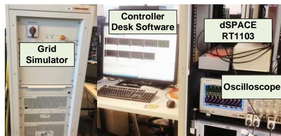
Fig. 9. Experimental Set up for real time implementation of the proposed technique.
