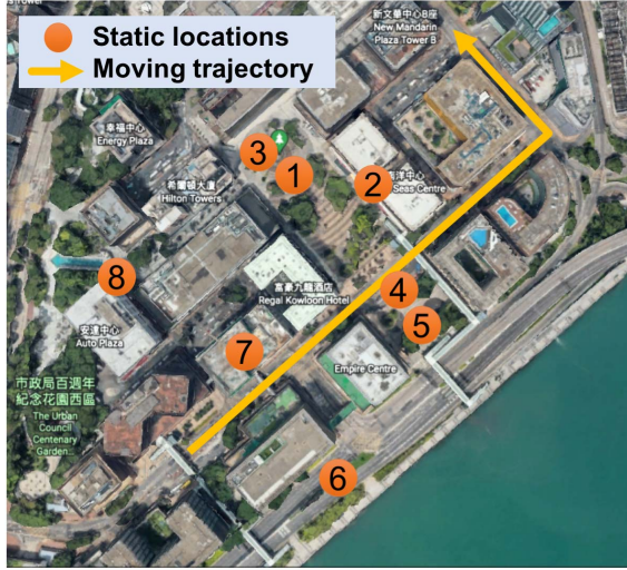
Fig. 2. Eight static locations (in orange) and one moving trajectory (in yellow) for GNSS data collection in Hong Kong urban canyon (around latitude 22.299° and longitude 114.177°).
