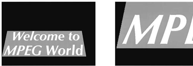
Fig. 1. An  $\alpha$ -plane image from test sequence Logo. Left) Full frame having 21 different pixel values. Right) Enlargement of part of the frame.
