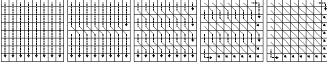
(a) First five out of sixteen 1-D transforms are shown. Each arrow indicates a 1-D DCT on the tranversed pixels. Remaining eleven transforms are symmetric versions.
