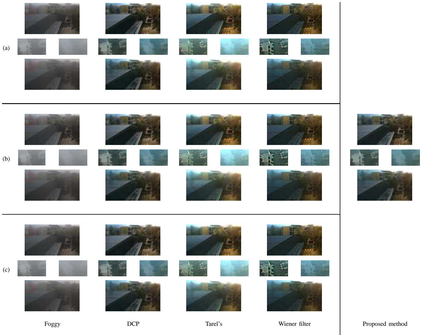
Fig. 10. Comparisons of joint defogging and demosaicking with denoised outputs in different foggy conditions. The comparing results were processed by the processing order of a typical pipeline—demosaicking, denoising, and defogging. The input foggy images are demosaicked by DLMMSE method. (a) Denoised output images by NLMM. (b) Denoised output images by BM3D. (c) Denoised output images by EPLL.
