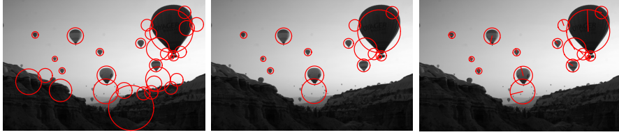
Figure 7: The different steps of the shearlet blob detector algorithm. Left: feature point localization; Centre: edge response elimination; Right: orientation assignment
