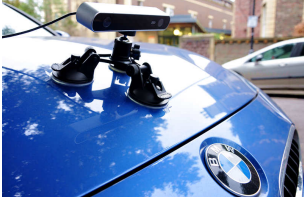
Fig. 10. Experimental set-up for acquiring stereo road images.
