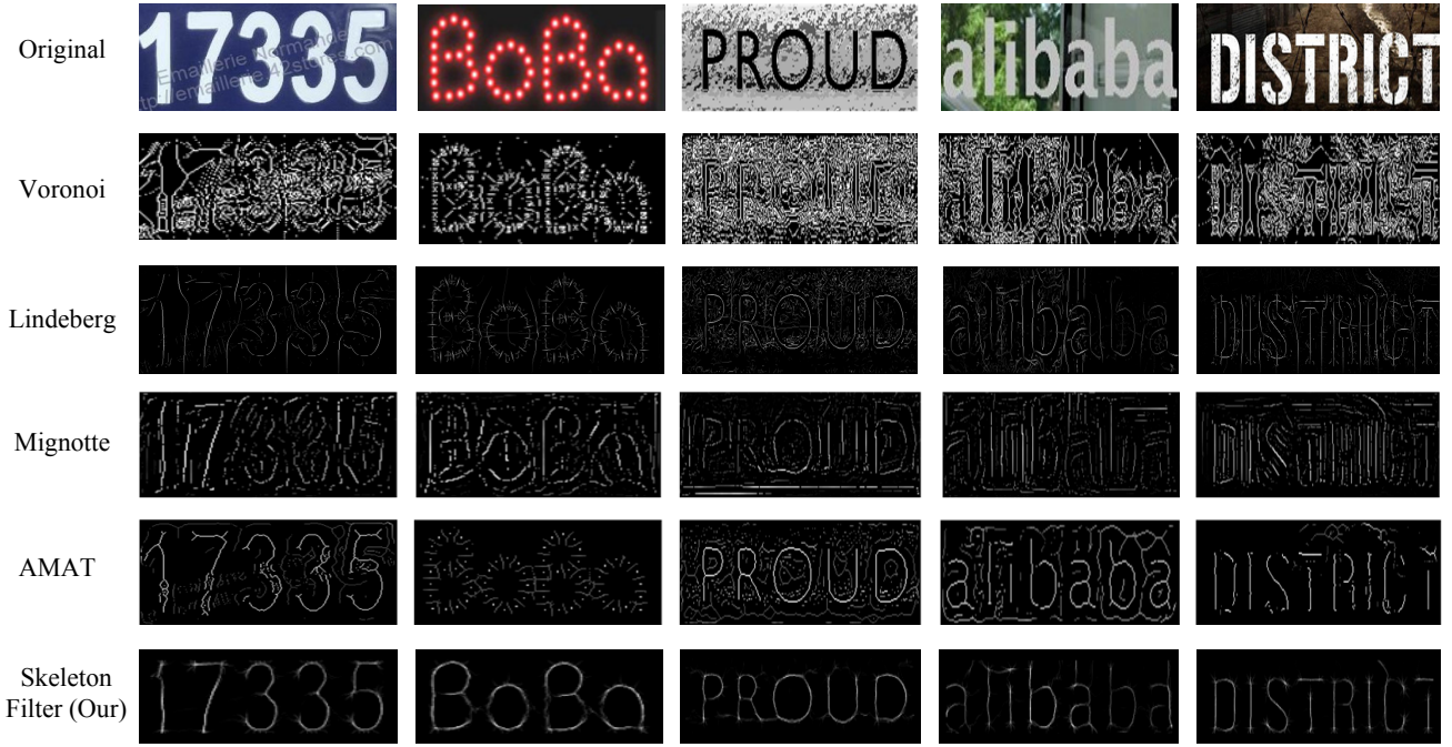
Fig. 8. Skeleton detection results on IIT5k. Skeleton detection methods include Voronoi, Lindeberg’s method, Mignotte’s method, AMAT and our Skeleton Filter. Here, the distance transform and thinning methods are less effective.
