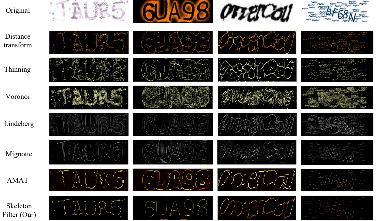
Fig. 6. Skeleton detection results on CAPTCHA. From left to right: BotDetect (2nd, 3rd columns), reCAPTCHA (4th column) and Paypal (5th column) datasets. Skeleton detection methods include Distance transform, Thinning, Voronoi, Lindeberg's method, Mignotte's method, AMAT and our Skeleton Filter.
