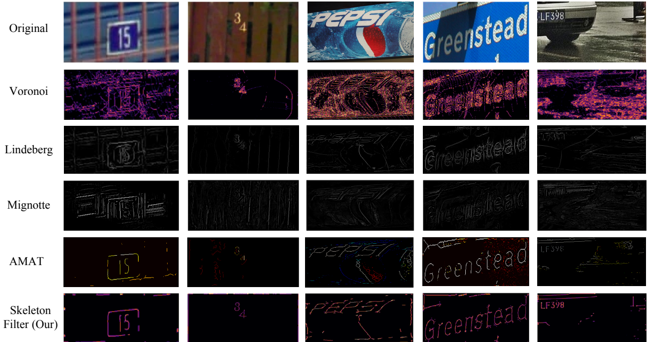
Fig. 7. Skeleton detection results on the natural scene text. From left to right: SVHN (2nd and 3rd columns) and ICDAR 2013 (4th and 5th columns) datasets in the natural world. Skeleton detection methods include Voronoi, Lindeberg's method, Mignotte's method, AMAT and our Skeleton Filter. Here, the distance transform and thinning methods are less effective.
