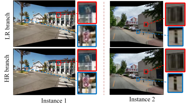
Fig. 7. The outputs of the low-resolution branch and high-resolution branch. The high-resolution branch is designed to enhance the resolution and refine the stitched image.
