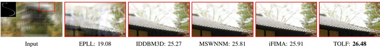
Fig. 7. Image restoration results on a challenging color image with a large-sized kernel ( $75 \times 75$ ). The PSNR score is reported below each subfigure.
