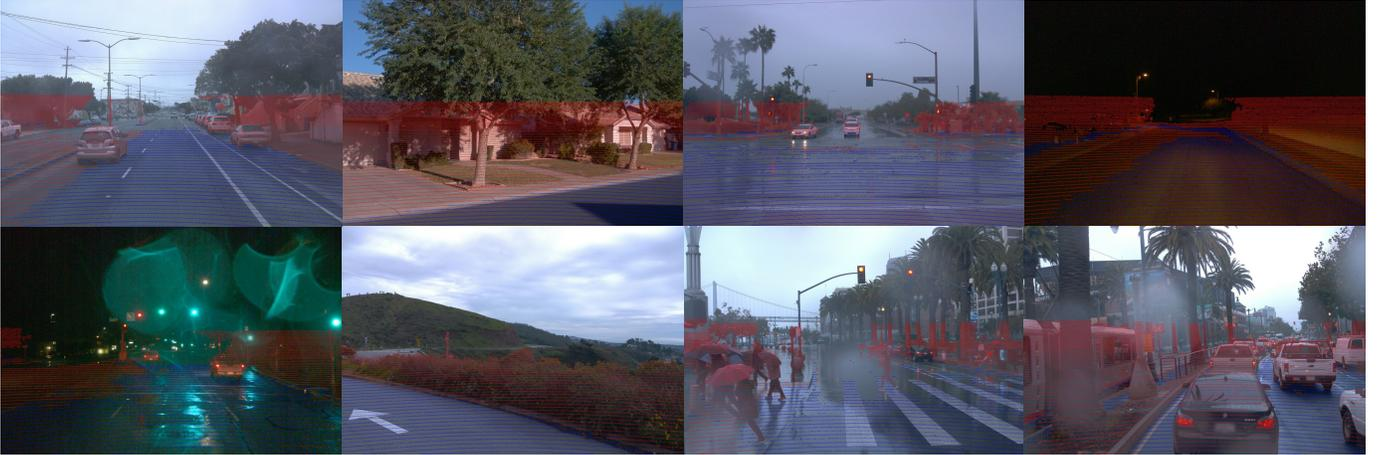
Fig. 4. The Waymo Open Dataset used to construct RP2-Waymo dataset. The points in the figures are the LiDAR used for constructing the dataset. The blue points are the points labeled with road. The road plane is extracted based on these points. Among all of the images, despite time, weather, scene vary, the road plane can be considered as a reference for planar parallax estimation.
