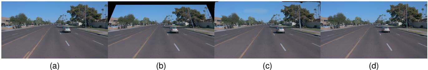
Fig. 7. (a) Source image  $I_s$ . (b) Homography warped source image  $I_s^w$ . (c) Reconstructed image  $I_t'$ . (d) Target image  $I_t$ . (a) to (b) refers to the homography aligning process; (b) to (c) refers to the planar parallax reconstruction process; (c) to (d) illustrates the difference between reconstructed image and the target image.
