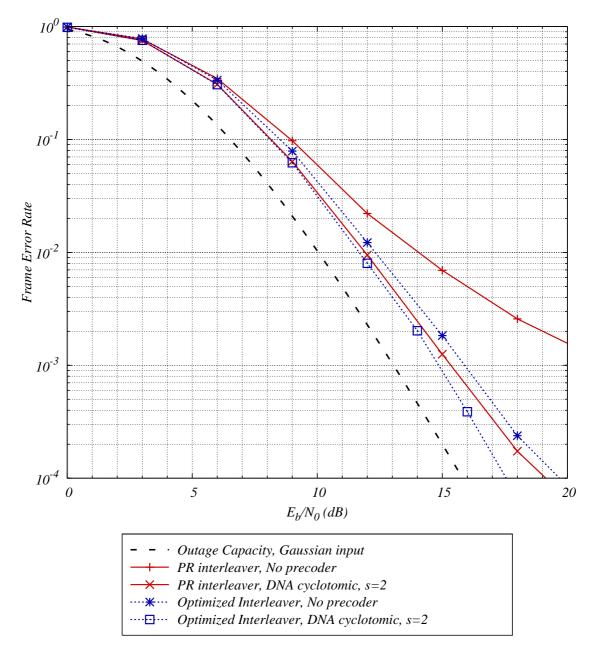
Figure 9: Optimized interleaver with rate-1/2 RSC  $(7,5)_8$  turbo-code and DNA cyclotomic precoder - 16-QAM,  $1 \times 1$  MIMO channel,  $n_c = 4$ , 15 iterations,  $L_c N_c = 2048$  - Parity check bits of the second constituent are multiplexed via the inverse turbo interleaver.
