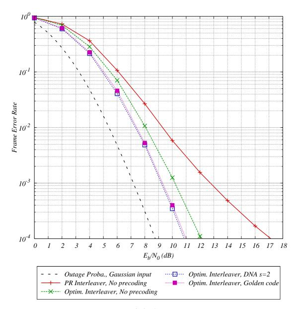
Figure 7: Optimized interleaver with rate-1/2 (7,5)<sub>8</sub> NRNSC code and linear precoders - QPSK,  $2 \times 2$  MIMO channel,  $n_c=2$ , 5 iterations,  $L_cN_c=256$  - No linear precoder, DNA cyclotomic precoder ( $s=2,n_s=1$ ), Golden code ( $s=2,n_s=1$ ).
