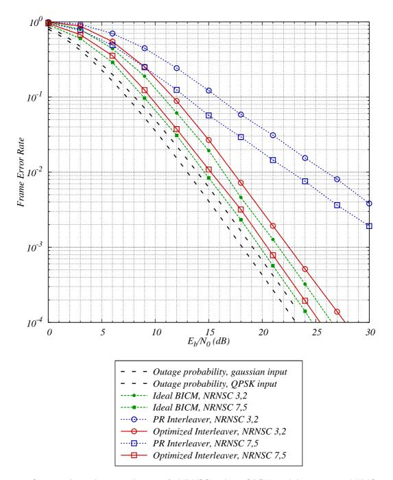
Figure 6: Optimized interleaver with rate-1/2 NRNSC codes - QPSK modulation,  $2 \times 1$  MIMO channel,  $n_c = 1$ , 10 iterations,  $L_c N_c = 1024$ .
