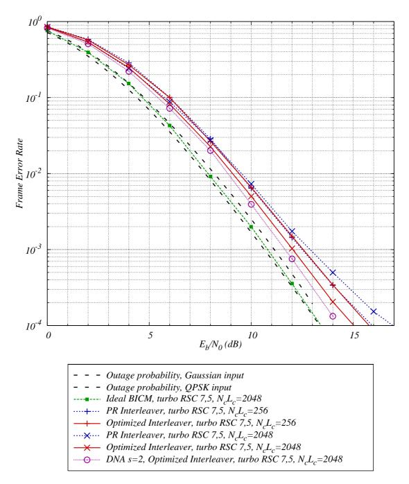
Figure 10: Impact of frame size with a rate-1/2 RSC  $(7,5)_8$  turbo-code - QPSK,  $2 \times 2$  MIMO channel,  $n_c = 1$ , 15 iterations - Parity check bits of the second constituent are multiplexed via the inverse turbo interleaver.
