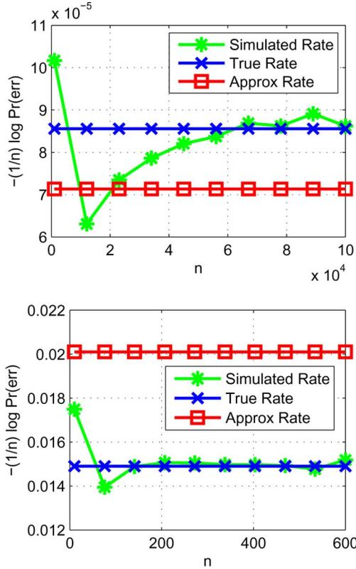
Fig. 11. Comparison of true, approximate and simulated rates with  $\gamma = 0.01$  (top) and  $\gamma = 0.2$  (bottom). Here the number of runs  $M = 10^7$  for  $\gamma = 0.01$  and  $M = 5 \times 10^8$  for  $\gamma = 0.2$ . The probability of error is computed dividing the total number of errors by the total number of runs.
