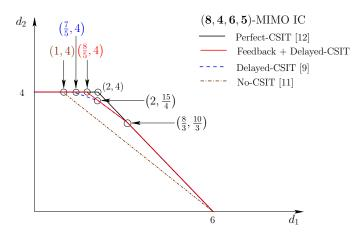
Fig. 4. DoF region for the (8, 4, 6, 5)-MIMO-IC with various assumptions.
