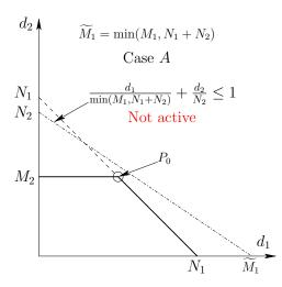
Fig. 5. Two cases for the  $(M_1, M_2, N_1, N_2)$ -MIMO-IC.
