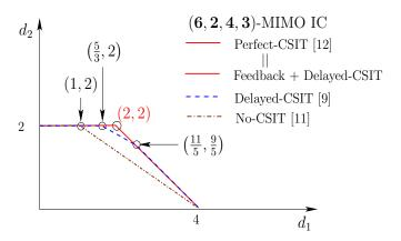
Fig. 2. DoF region for the (6, 2, 4, 3)-MIMO-IC with various assumptions.
