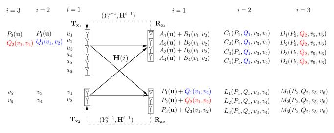
Fig. 3. Coding scheme with FB and delayed CSIT: (6, 2, 4, 3)-MIMO-IC.
