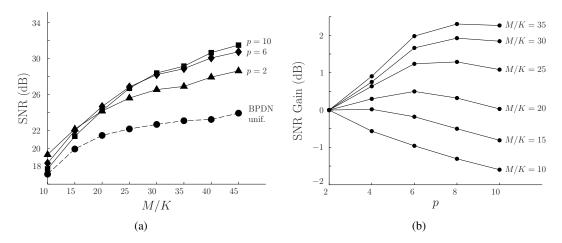
Fig. 3: Reconstruction SNR of GBPDN( $\ell_{p,w}$ ). (a): the dashed line represents the reconstruction quality achieved from uniformly quantized CS and BPDN. (b) SNR gain versus p for each tested oversampling ratio M/K.
