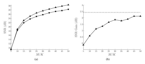
Fig. 2: Stabilized versus unstabilized reconstruction using GBPDN( $\ell_{2,w}$ ) and BPDN respectively. (a) The reconstruction SNR using stabilized (triangles) and unstabilized (squares) methods. (b) Observed (triangles) and theoretically predicted (dashed) SNR gain at 2.43 dB brought by stabilization.
