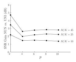
Fig. 5: Reconstruction gain (in dB) between non-uniform or uniform quantization at the same p.
