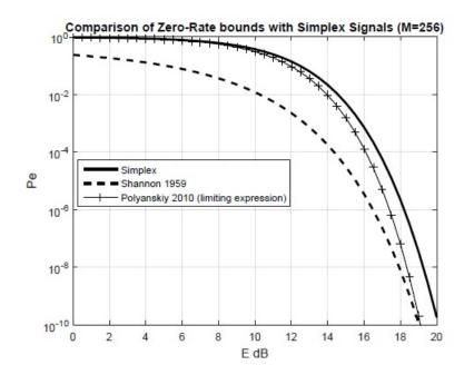
Fig. 2: Comparison of Zero-Rate Bounds with the error-probability of a Simplex (M = 256)
