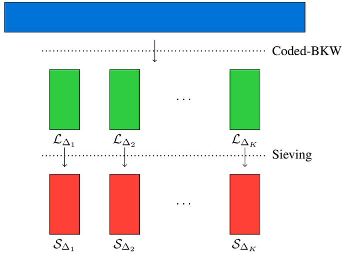
Fig. 2. A macro picture of how one step of coded-BKW with sieving works. The set of lists  $\mathcal{S}_{\Delta_1}, \dots, \mathcal{S}_{\Delta_K}$  constitutes the samples for the next step of coded-BKW with sieving.
