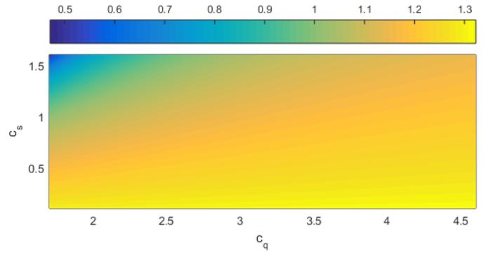
Fig. 6. The optimal  $\gamma$  value for version D of the algorithm, as a function of  $(c_q, c_s)$ .
