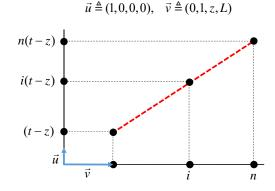
Fig. 3. Linear relationship between the maximal length of the file that can be stored and the three resources key length, local randomness, and public communication. For instance, for  $i \in \mathbb{N}$ , storing a file of i(t - z) bits requires *i*-bit keys,  $i \times z$  bits of local randomness, and  $i \times L$  bits of public communication.
