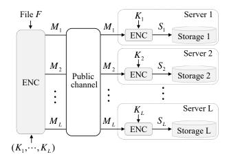
Fig. 2. In our setting, individual and information-theoretically secure channels between each server and the user are replaced by a public communication channel and pairs of secret keys between the user and the servers. One of our main objectives is to characterize the minimum key lengths needed for a given file size.
