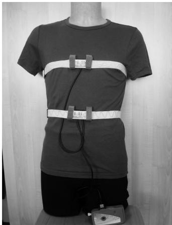
Fig. 2. Vitaport CPS system along with the two belts containing the inductive coils.
