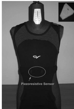
Fig. 4. MyHeart shirt with the piezoresistive sensor highlighted by a circle. In the upper right corner, the PPU is shown.
