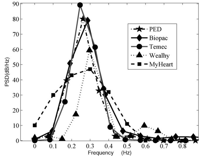
Fig. 8. FFTs of a simple respiration activity acquired by all the systems over the same time interval.
