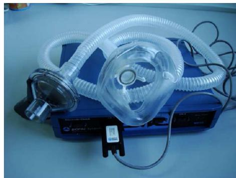
Fig. 1. Biopac system used as spirometer along with the facemask.
