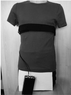
Fig. 5. Belt containing the piezoelectric sensor.
