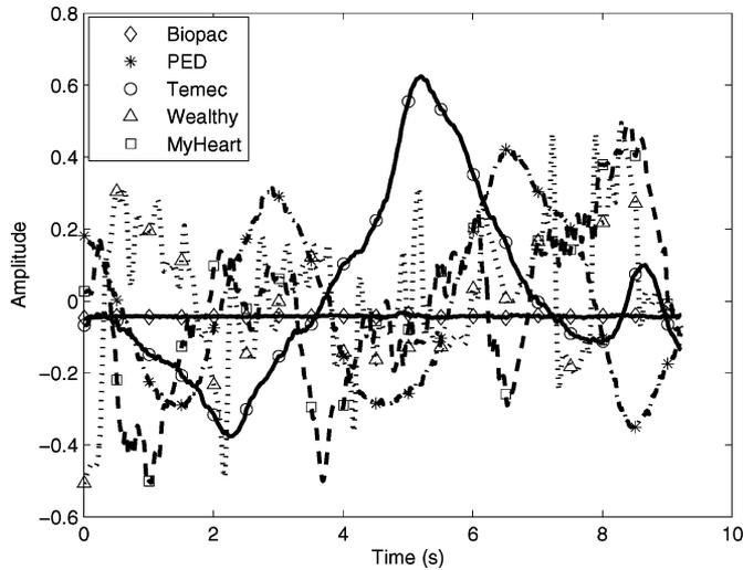
Fig. 6. Output signals over time from all the systems, included the spirometer, during a physical exercise without breathing.
