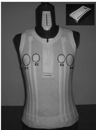
Fig. 3. Wealthy shirt. E1 and E4 are the electrodes used to inject current and E2 and E3 are used to acquire the voltage drop. Dividing the voltage by the current, we can obtain the transthoracic electric impedance. In the upper right corner, the PPU is shown.
