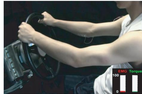
Fig. 4. Experimental condition for the measurements of human impedance properties in steering by the arms.
