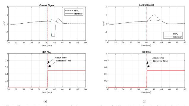
Fig. 4. The intelligent intrusion detection system output for the two covert attack scenarios. The attack time is t=40 and the detection time is not much later than the attack time. (a) The first attack scenario. (b) The second attack scenario.
