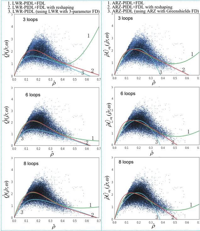
Fig. 8. Comparison of the FD curves estimated by the PIDL+FDL-based TSE methods and PIDL-based TSE methods. For consistent visualization, the learned  $\hat{U}_{eq}(\hat{\rho}; \omega)$  is converted to  $\hat{\rho}\hat{U}_{eq}(\hat{\rho}; \omega)$  to represent the estimated flow.
