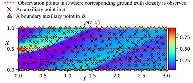
Fig. 2. A sparse presentation of the deployment of observation points  $O$  at loop detectors, auxiliary points  $A$  randomly selected from  $G$ , and boundary auxiliary points  $B$  deployed at the boundaries  $x = 0$  and  $x = 1$  for certain time points. The heatmap is the numerical solution of Eqs. (9) using the Godunov scheme. We treat the numerical solution as the ground truth.
