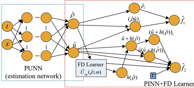
Fig. 5. PIDL+FDL architecture for second-order traffic dynamics. The model parameter  $\tau$  is held by a variable node (blue rectangular node).
