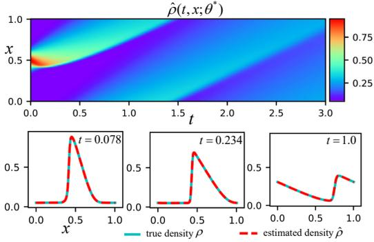
Fig. 3. Top: Estimation of the traffic density dynamics  $\hat{\rho}(t, x; \theta^*)$  on grid points  $G$  in the domain using the trained PUNN. Bottom: Snapshots of estimated and true traffic density at certain time points.
