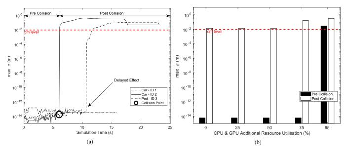
Fig. 7. Vehicle to pedestrian collision (Test 4) showing (a) maximum deviation against simulation time for 25% resource utilisation and (b) maximum deviation pre- and post-collision for different resource utilisation levels.
