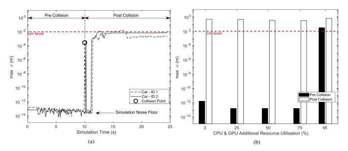
Fig. 6. Vehicle to vehicle collision (Test 2) showing (a) maximum deviation against simulation time for 25% resource utilisation and (b) maximum deviation pre- and post-collision against resource utilisation. The simulation noise floor is shown in (a) which is the empirical lower limit of deviation for the hardware reported in this study.
