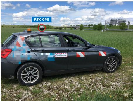
Fig. 14. This is our test car with high-precision RTK-GPS device (cm-level).
