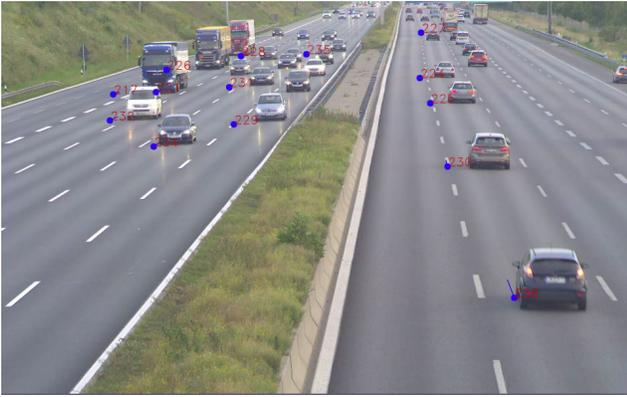
Fig. 2. This is the image after the traffic radar measurements being projected onto the camera picture. The measurements (blue points) are sparse, and contain biases and misdetections caused by noise.
