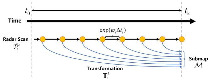
Fig. 5. This diagram shows the radar sub-map construction pipeline. We can obtain a dense radar sub-map  $\mathcal{M}$  by aggregating radar scans  $\hat{\mathcal{P}}_i^c$  between  $t_0$  and  $t_k$ . The transformation matrix  $\mathbf{T}_i^k$  can be obtained by integrating instantaneous ego-velocities  $\varpi_i$  in a short period  $\Delta t_i$ .
