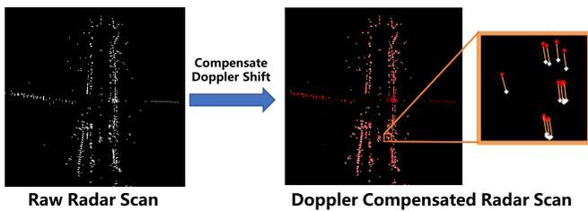
Fig. 4. This diagram shows the Doppler compensation operation with a zoomed-in view. The Doppler compensation is performed in each radar scan to restore the Doppler distortion. The radar scan after compensation is highlighted in red. The orange lines represent the range shift  $r_d$ .
